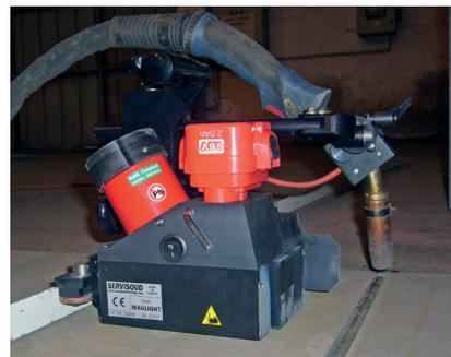
▲ Sheet metal butt welding
